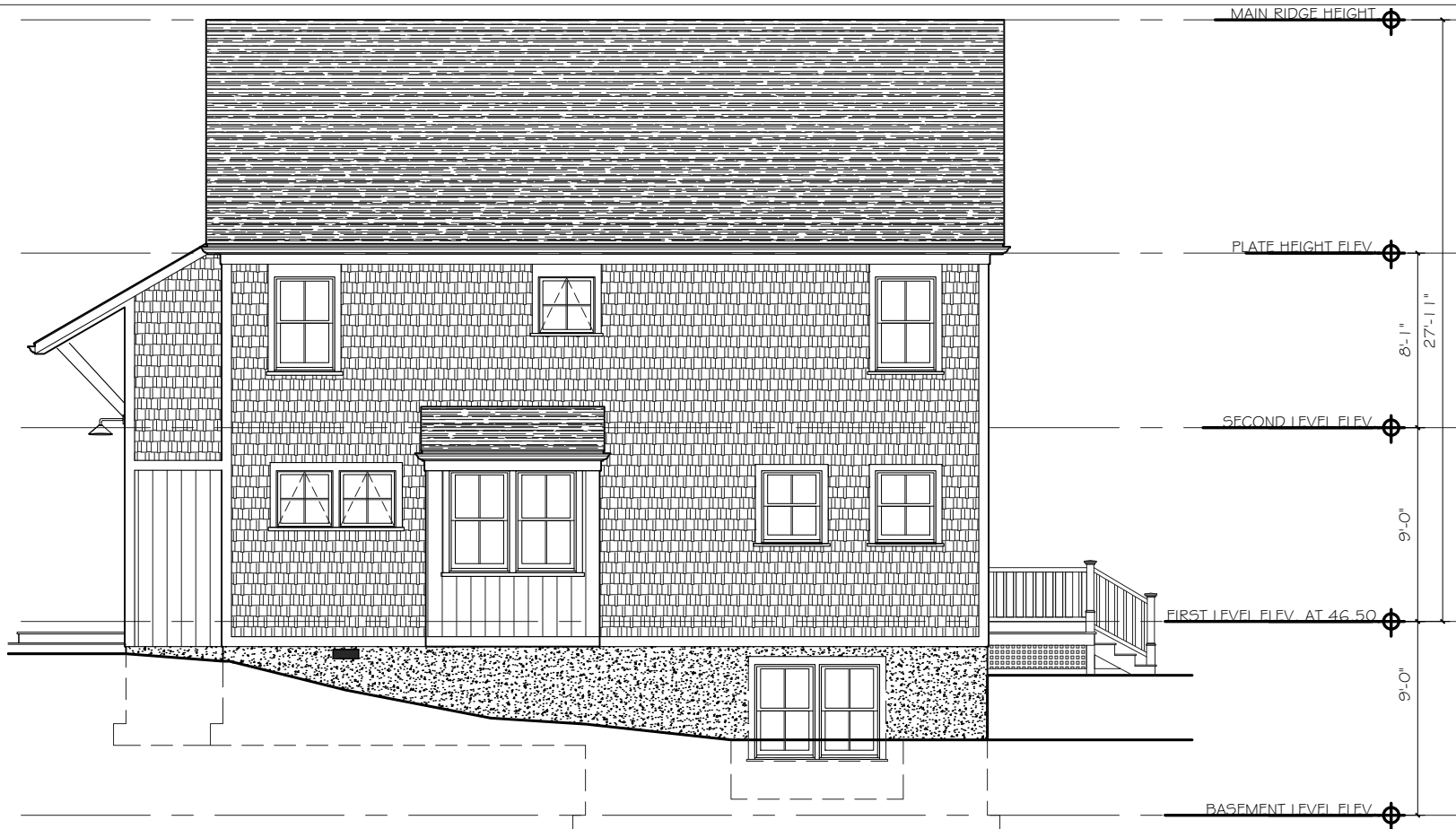
② SIDE ELEVATION 1 (SIDE MAY BE MIRRORED DEPENDING ON THE BUILDING) SCALE: 1/8" = 1'-0"
