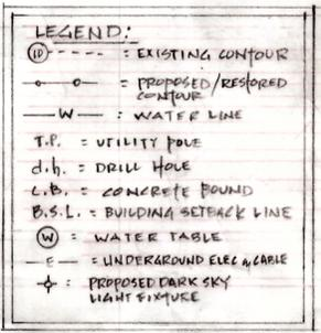
NOTE: LIMIT OF WORK ARE THE EAST & WEST PROPERTY LINES AT ALONG BOTTOM OF OLD SLOPE LINE AND IN FRONT OF ROCKS - CONTRACTOR TO STAKE STRAW BALES AT SLOPE FENCE ALONG PROPERTY LINES & BOT. OF SLOPE AND MAINTAIN SAID LIMIT OF WORK DURING CONSTRUCTION.
