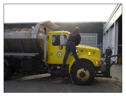
Employee safety is compromised when trying to clear off large equipment in inclement weather conditions as shown above
