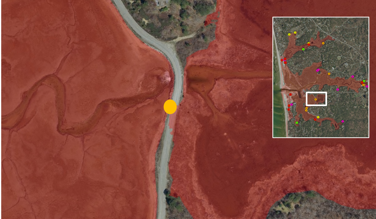
Figure 7. Example of Inundation Pathway-Road (IP-R). The red represents the approximate extent of water during an inundation event. This pathway only leads to flooding along the road, however it is a critical route for emergency vehicles.
