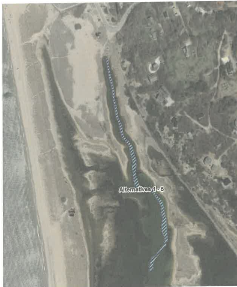
Figure 5. Portion of outlet channel to Pamet Harbor identified for improvement to better drain Little Pamet River (included with Alternatives 1 through 5).
