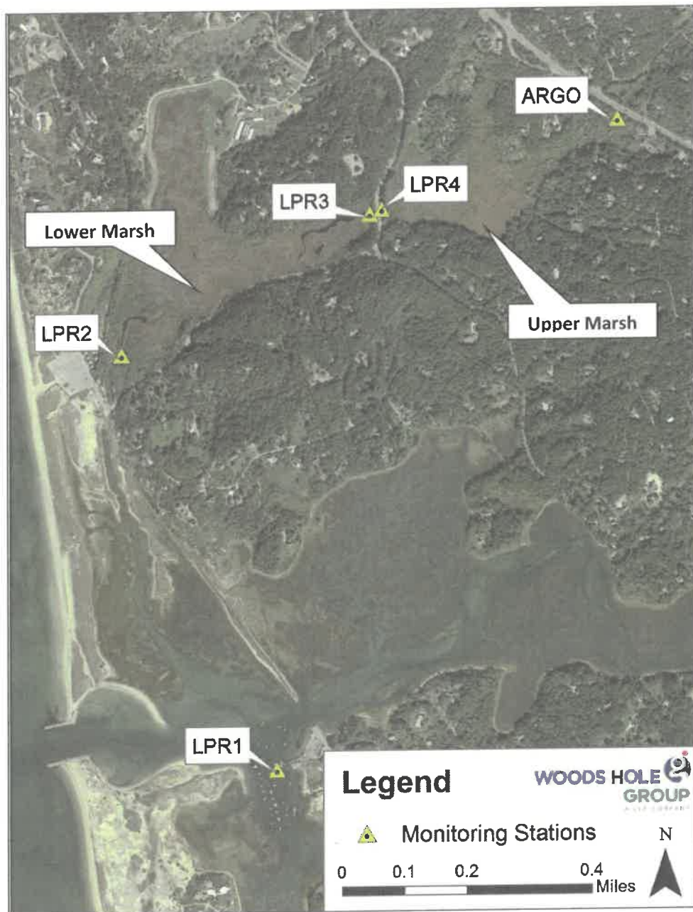
Figure 1. Locus map of the Little Pamet River estuarine system. Call out boxes indicate the different reaches of the system and approximate locations of the AquaTroll data loggers and Argonaut current meter deployed in support of this study.
