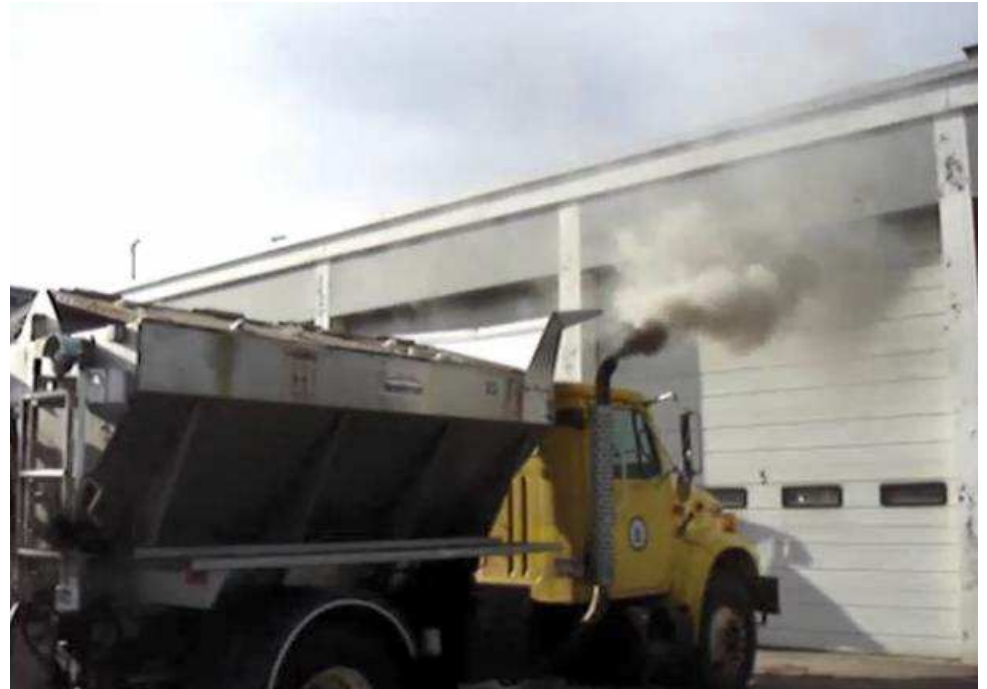
Vehicle starting when stored outdoors Excessive exhaust due to cold engine start
