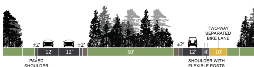
Figure 9 - Alternative 2 cross sections.
