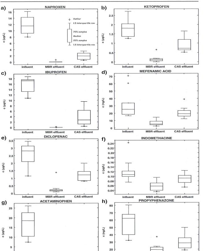
Fig. 1 Removal, during MBR and CAS treatment, of the analgesics and anti-inflammatory drugs naproxen (a), ketoprofen (b), ibuprofen (c), mefenamic acid (d), diclofenac (e), indomethacin (f), acetaminophen (g), and propyphenazone (h)
