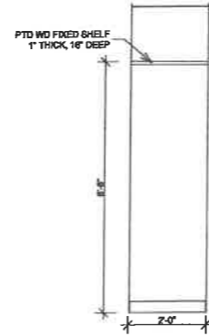
2 BROOM CLOSET (DOOR 120) LOOKING W SCALE: 1/2" = 1'-0"
