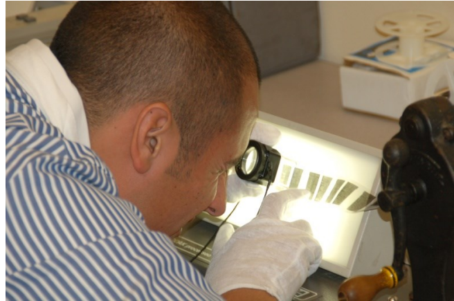
A Kofile Technician examines a roll of microfilm during a quality assurance assessment.
