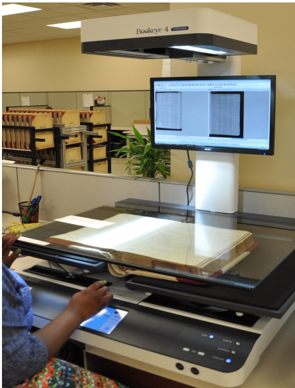
Bookeye® 4 Book Scanner for Bound Volumes in use at Kofile. This photograph illustrates the cradle positioned at 180° The spine of the volume is resting in the cradle.
