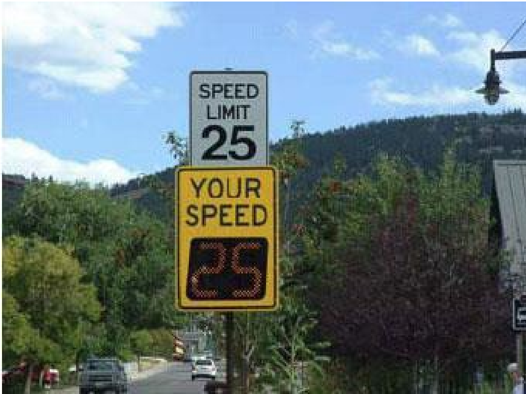
Figure 3.1 –Pole Mounted Speed Display Sign
