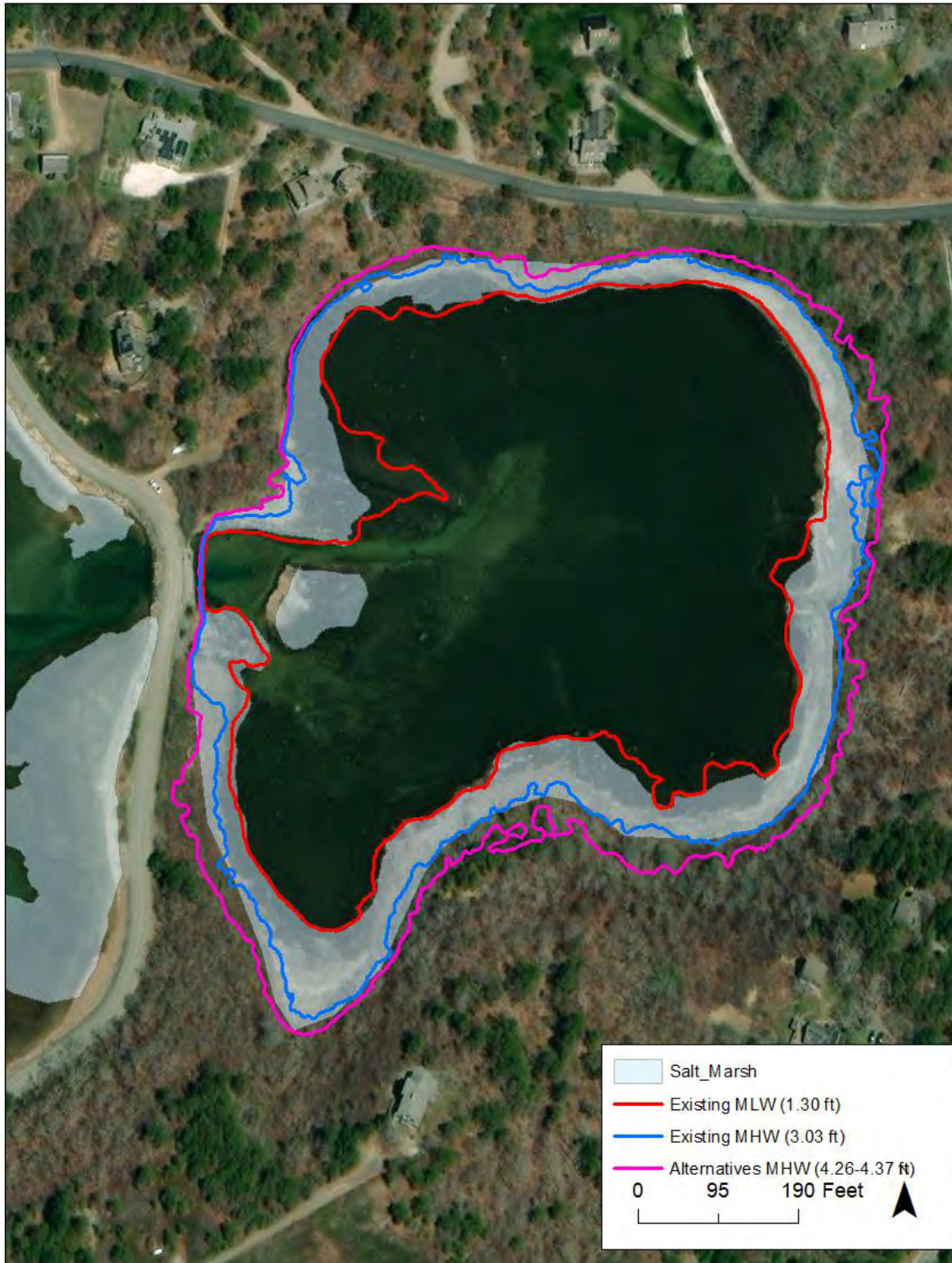
Figure 21. Comparison of the extent of existing salt marsh relative to MLW and MHW levels for existing conditions (red/blue) and the alternatives (pink).
