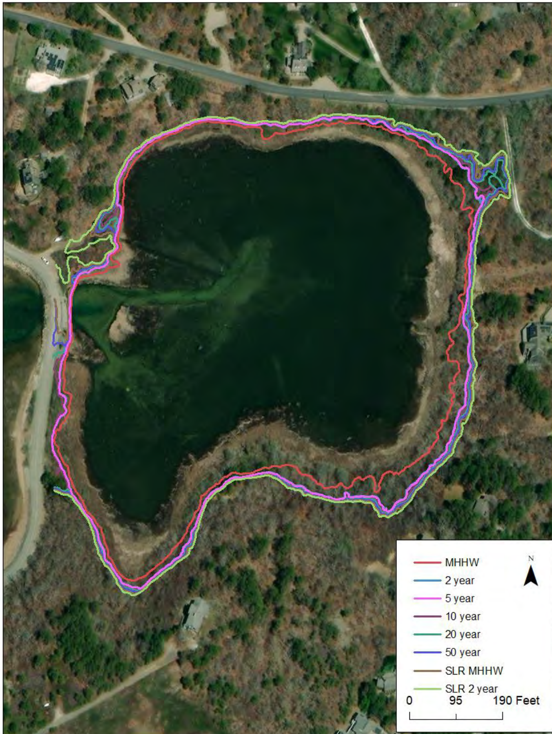
Figure 23. Comparison of the extent of existing salt marsh relative to MHHW and return period storms with and without sea level rise (SLR) for the alternatives modeling.
