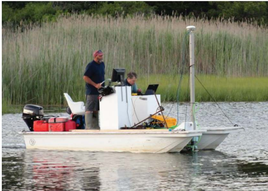
Figure 5. Provincetown Center for Coastal Studies pontoon boat for surveying shallow estuaries.
