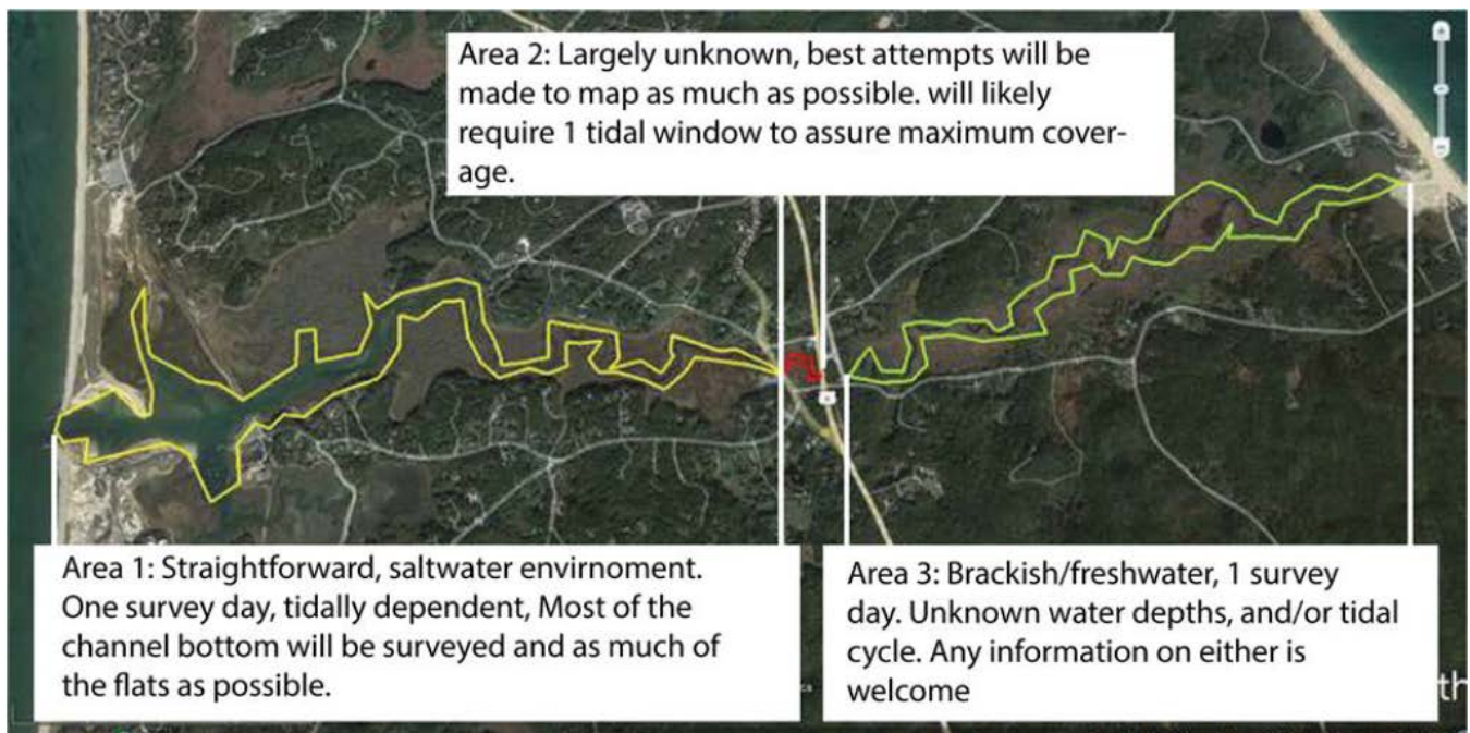
Figure 4. Approximate bathymetric survey extents of the Pamet River for the lower reach (yellow), middle reach between Truro Center Rd and Route 6 (red), and upper reach upstream of Route 6 to Ballston Beach.
