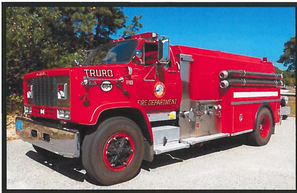
Figure 12 - Tender 484 – 1987 Tanker – GM Top Kick/Maxim, 500 GPM Pump, 2,0000 gallon tank - Acceptable Condition
