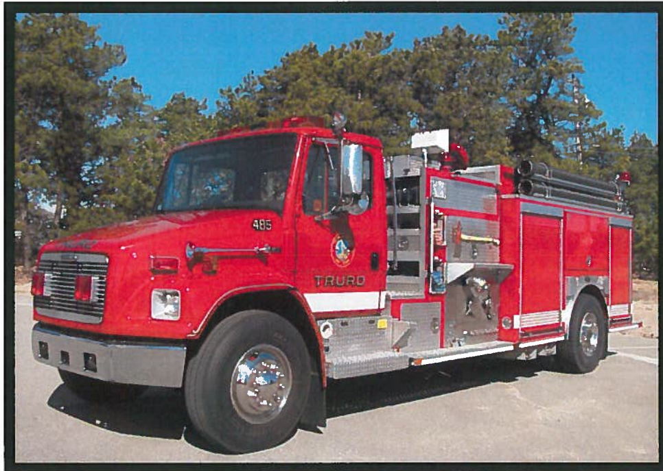
Figure 9 - Engine 485 – 197 Freightliner FL80/E-One Pumper, 1,500 GPM Pump, 40 gallons of foam - Good Condition
