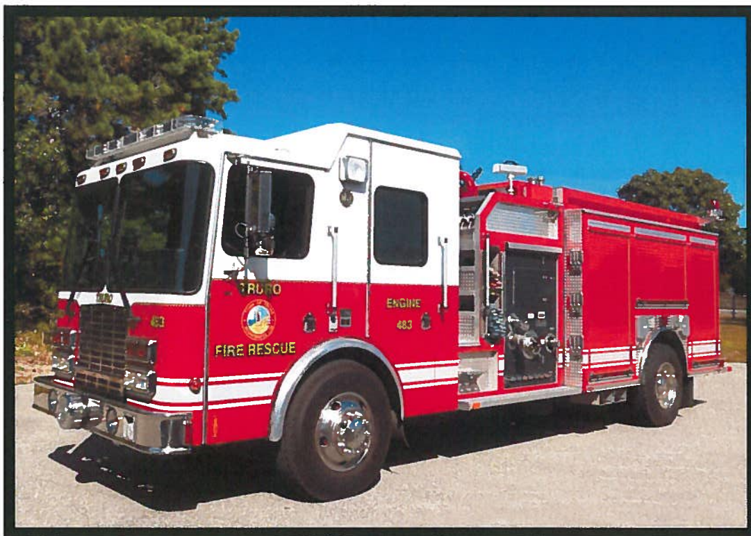
Figure 8 - Engine 483 – 2006 HME/Ferrara Pumper 1500 GPM Pump, 1,000 gallon tank – serves as a Structural Attack Engine - Good Condition
