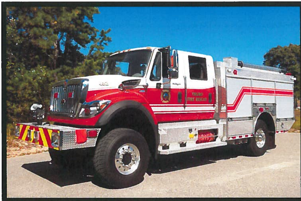
Figure 10 - Engine 482 – 2013 International/Rosenbauer Timberwolf AWD 1,250 GPM Pump, 750 gallon tank, 30 gallons of foam - Urban Interface Quick Response Unit - New Not in Service
