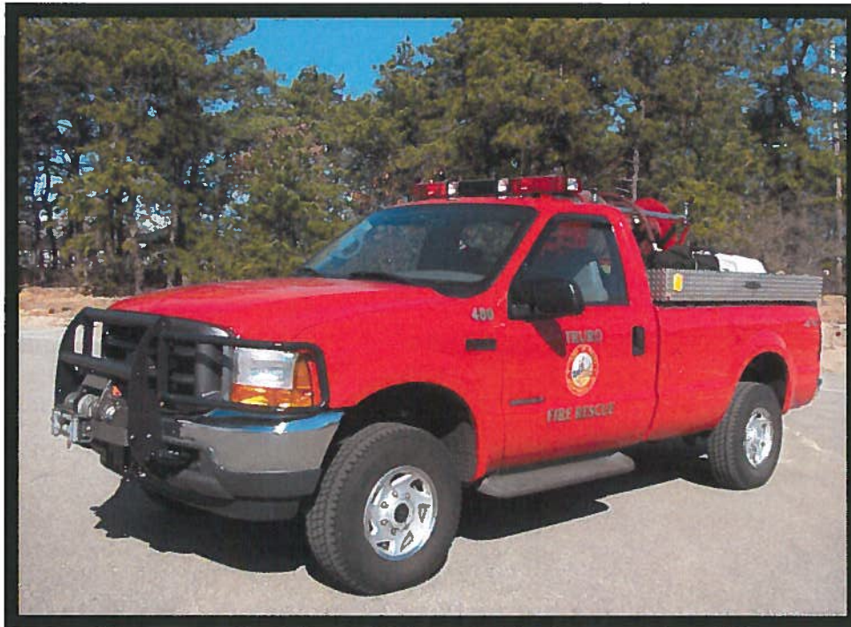
Figure 11 –Forestry 480 – 2001 Ford F 350 4X4 built by FireOne. 200 GPM Pump, 250 gallon tank - Good Condition
