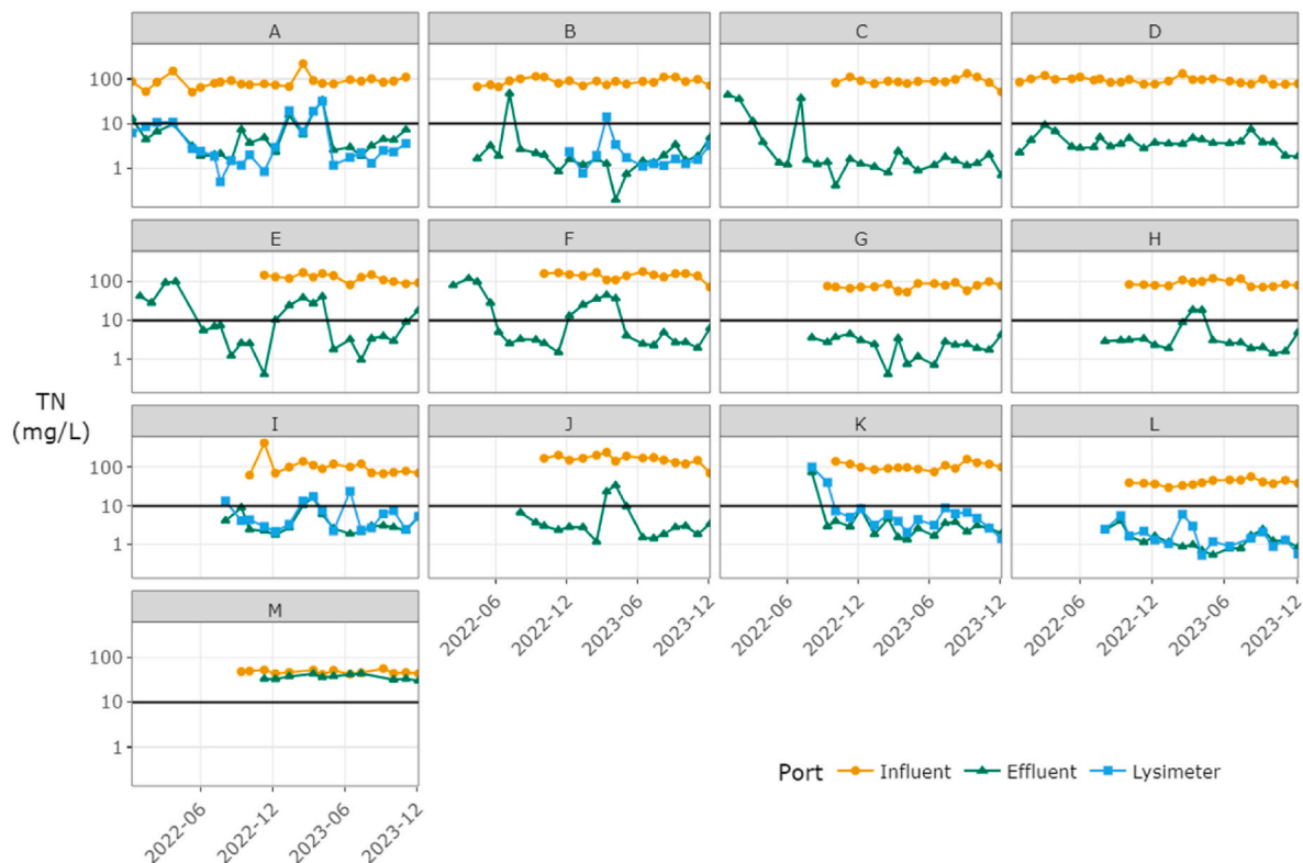
Fig. 5. Total nitrogen (TN) concentrations (mg/L) over time, by site and sampling port, in wastewater from 13 Innovative/Alternative septic systems in Barnstable (Cape Cod), Massachusetts, a cohort comprised of two models that incorporate woodchip bioreactors to enhance N removal. Note that the vertical axes have a logarithmic scale. The performance goal of 10 mg/L is indicated with a black line.
