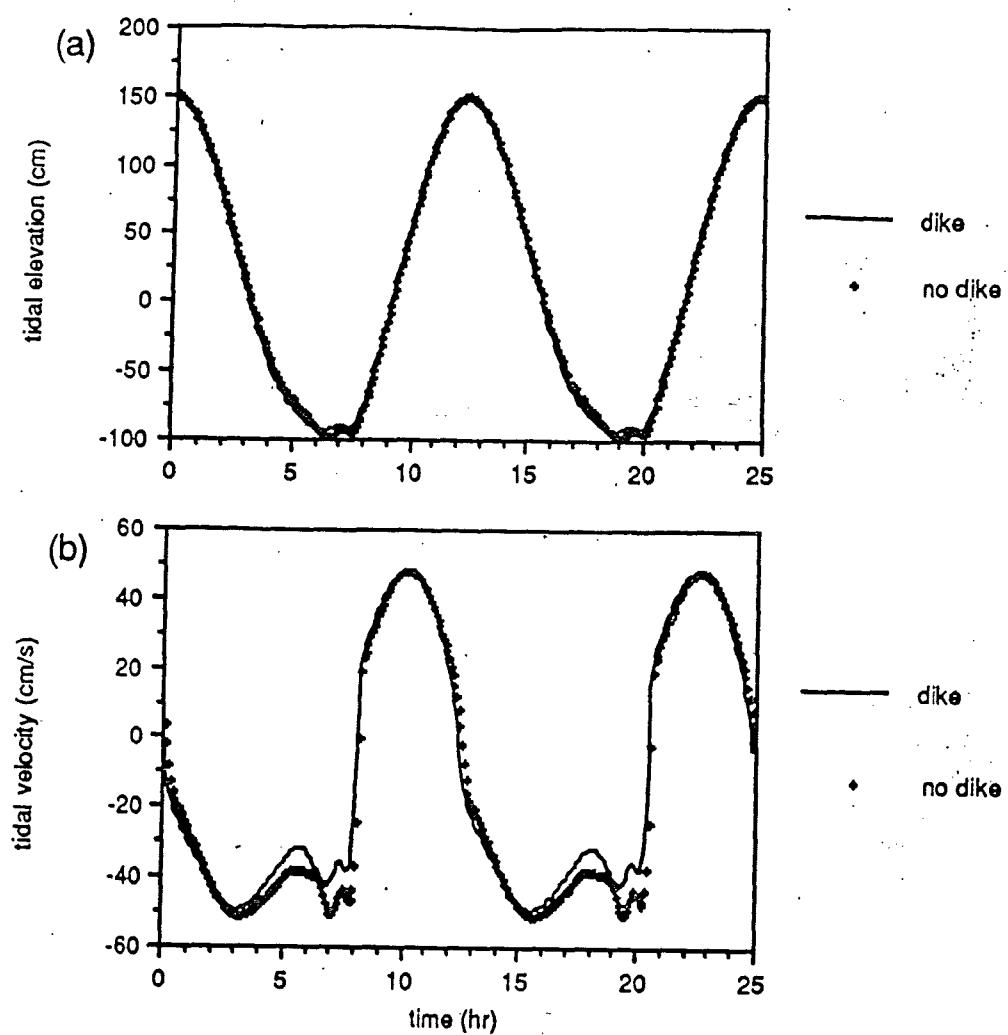
Figure 9. Comparison of modeled tides at inlet, with and without older Dike.
