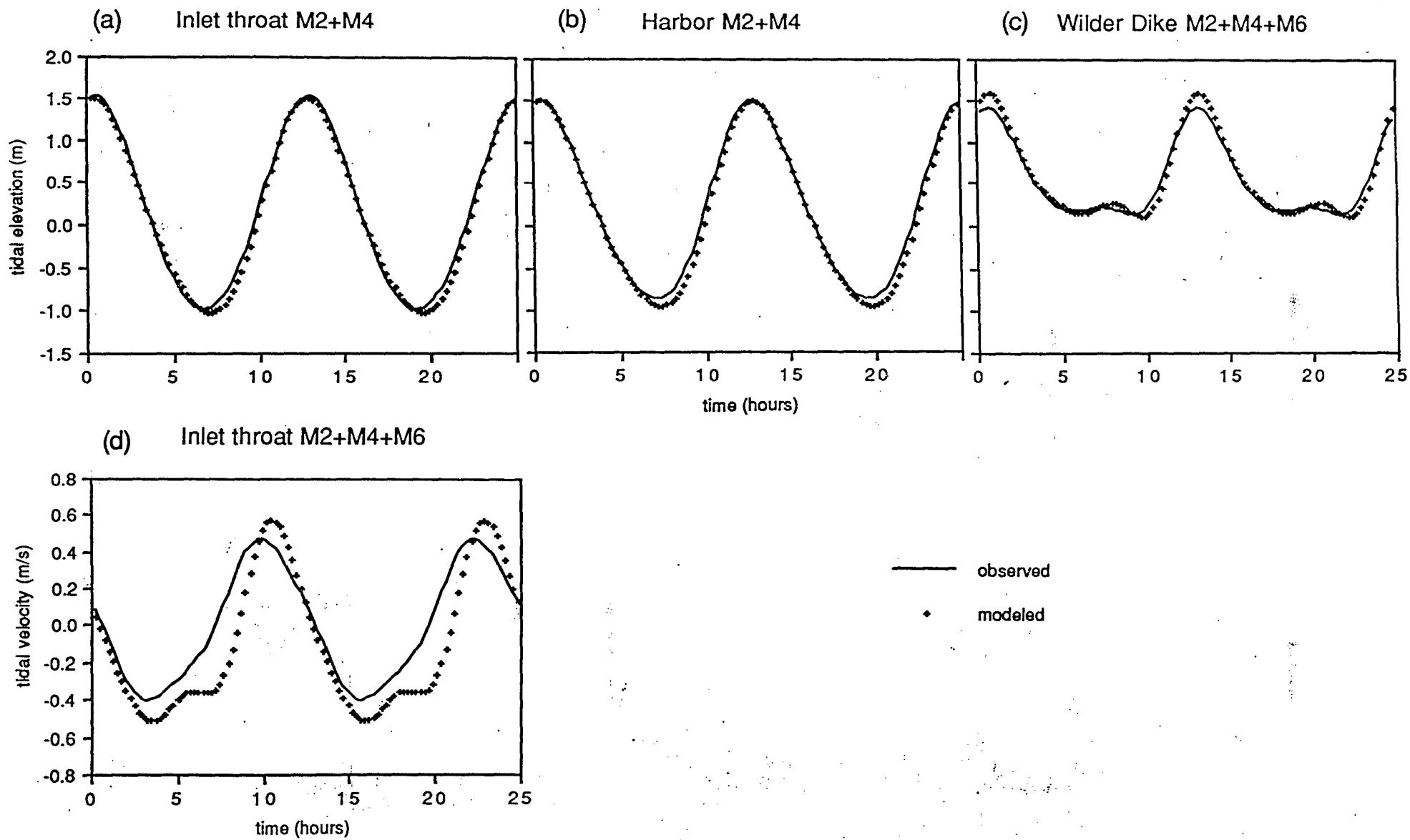
Figure 7. Reconstruction of tidal elevations and velocities from tidal harmonic constituents.
