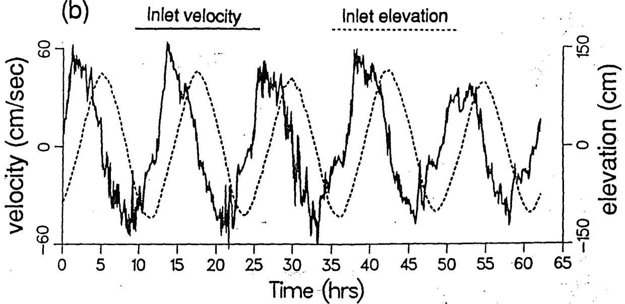
Figure 3. Field observation of Pamet River (a) tidal elevations at Cape Cod Bay, the harbor and Wilder Dike; and (b) tidal elevations and currents at the inlet.
