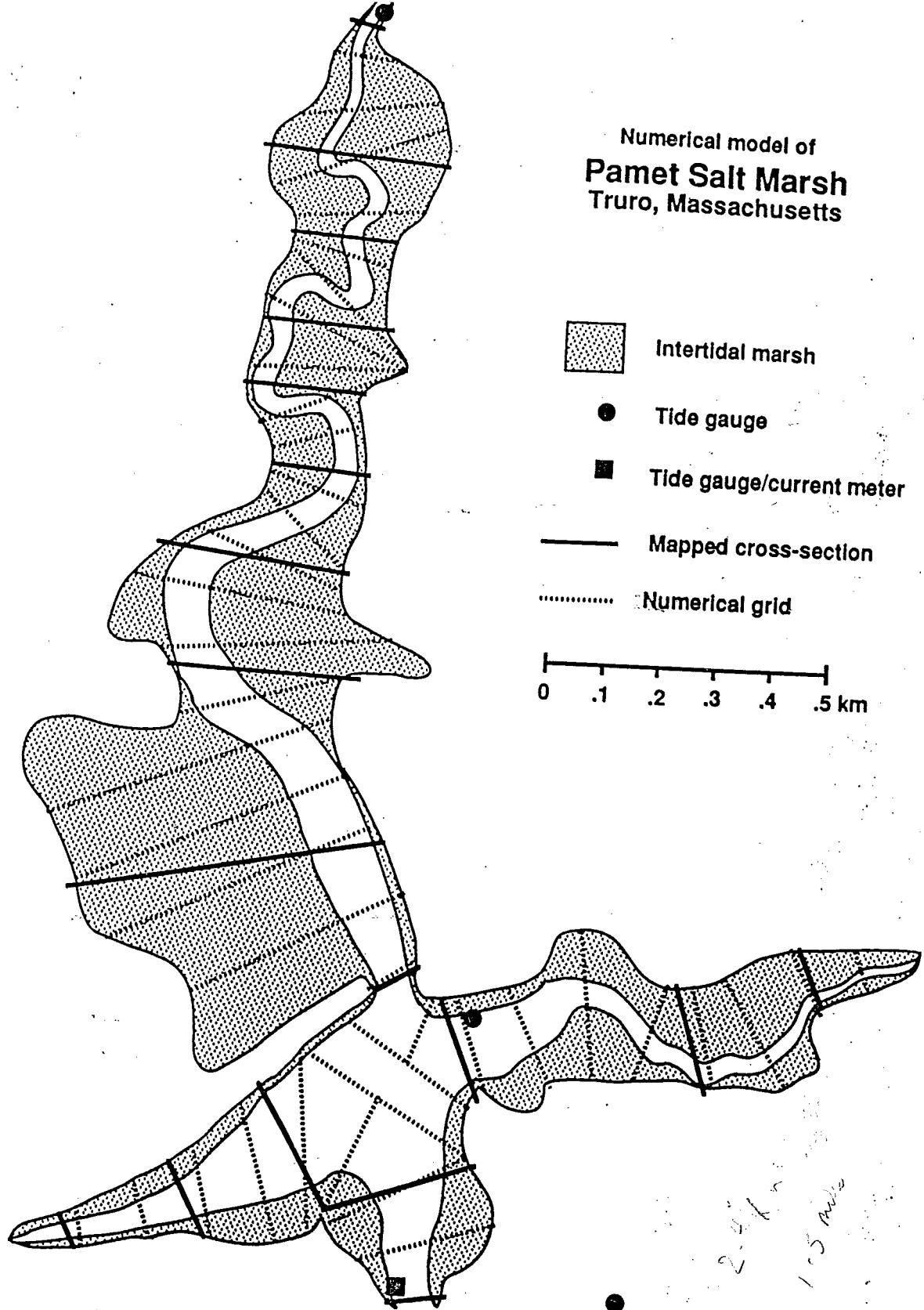
Figure 5. Plan of numerical model with locations of instrument stations and field-mapped cross-sections.
