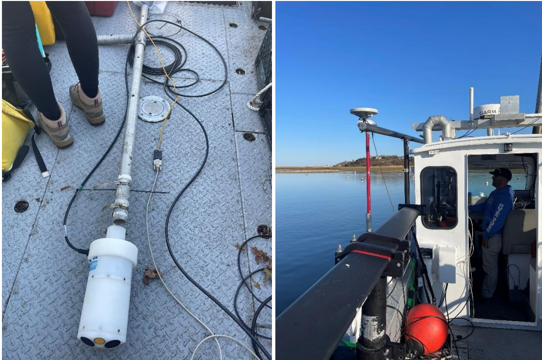
Figure 5a & 5b SonTek 1-MHz RiverSurveyor ADCP (left) and the vessel mount with RTK GPS integration (right).
