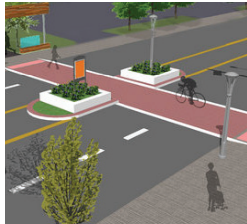
Pedestrian refuge island http://www.mlive.com/news/ann-arbor/index.ssf/2013/10/yp-silanti_to_construct_pedestr.html
