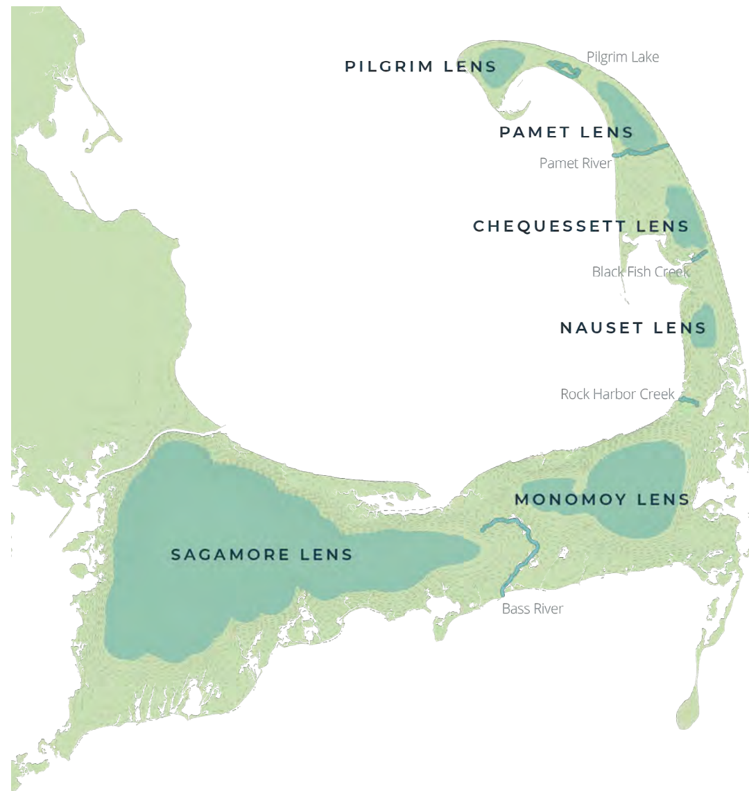
Figure 2. The six distinct groundwater lenses on Cape Cod and the low-lying bodies of water that separate them.
