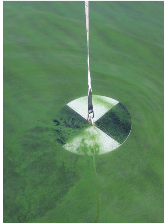
A Secchi disk is used to measure transparency depth. Photo sourced from United States Geological Survey.
