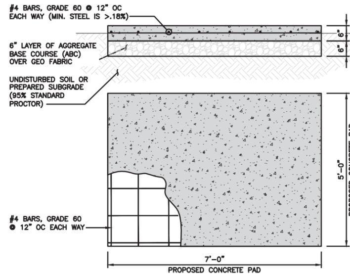
**TYPICAL CONCRETE PAD DETAIL**
