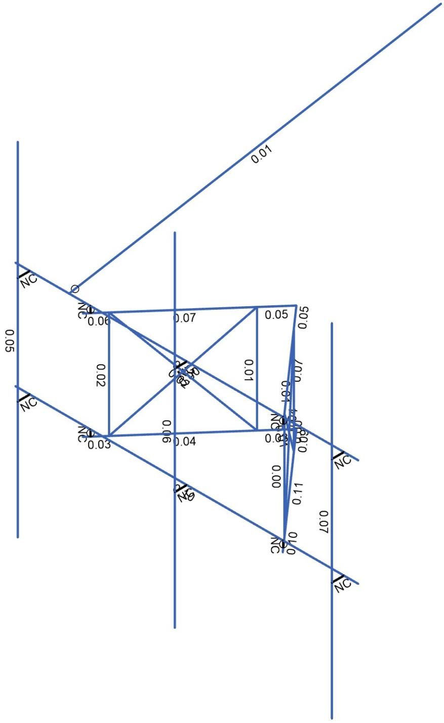
Member Shear Checks Displayed (Enveloped)
