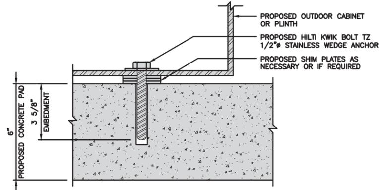
**TYPICAL OUTDOOR EQUIPMENT TO CONCRETE SLAB ANCHORAGE**
